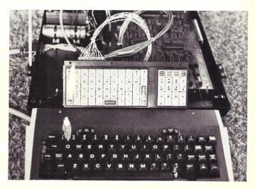
Internal keyboard detached to show how external keyboard is wired to it.
